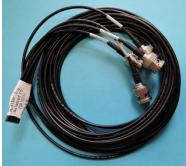
The monitor signals are fed out on an 8pin 2.54 mm post connector with two rows. Each monitor signal has its own ground pin. An adapter from the post connector to four BNC connectors is included (length 2 meters) – see photos left.
