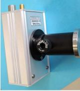
In the center at the bottom of the *BPD* an M4 mounting-thread (depth 6 mm) is available. Since this adapter is made out of plastic it electrically insulates the *BPD* housing from the optical table. The M4 thread allows attaching a metric post (e.g. ThorLabs TR30/M + PH40/M) for directly mounting the device on an optical table – see photos on the left.
