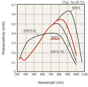
The absolute maximum power dissipation of the S5972 is specified with 50 mW. This corresponds to maximum 5 mA photocurrent at the applied bias voltage of 10 V. Then the optical power on the photodiode is 9.26 mW @800 nm. Since at the maximum power dissipation the photodiode may be damaged it is strongly recommended to work with optical power well below 4 mW.
