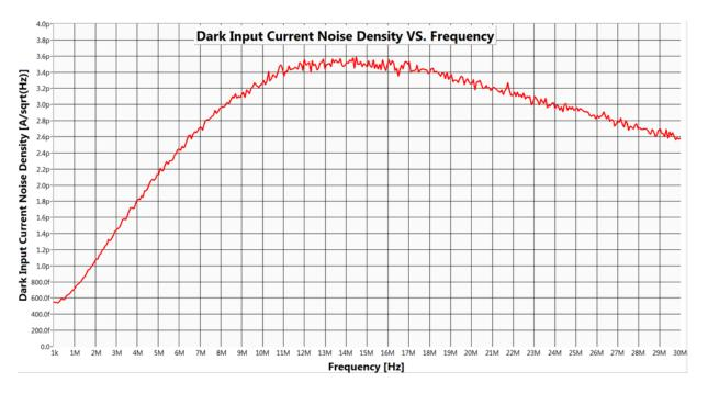
Light absorbed on a biased photodiode generates a leakage current which intrinsically carries shot noise. Given the DC leakage current through the photodiode ( $I_{DC}$  [A]) the shot noise current density ( $I_{shot}$  [A/VHz]) can be derived from ( $e_0$  = 1.602E-19 [As]):
