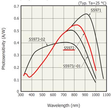
The absolute maximum power dissipation of the S5972 is specified with 50 mW. This corresponds to maximum 5 mA photocurrent at the applied bias voltage of 10 V. Then the optical power on the photodiode is 9.26 mW @800 nm. Since at the maximum power dissipation the photodiode may be damaged it is strongly recommended to work with optical power well below 4 mW.
