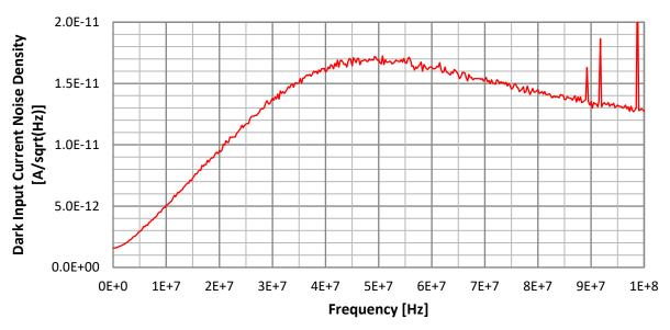
Light absorbed on a biased photodiode generates a leakage current which intrinsically carries shot noise. Given the DC leakage current through the photodiode ( $I_{DC}$  [A]) the shot noise current density ( $I_{shot}$  [A/VHz]) can be derived from ( $e_0$  = 1.602E-19 [As]):
