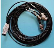
The monitor signals are fed out on an 8pin 2.54 mm post connector with two rows. Each monitor signal has its own ground pin. An adapter from the post connector to four BNC connectors is included (length 2 meters) – see photos left.
