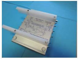
2. Switch off the LNHR DAC and attach the six BNC plug-to-plug adapters on the channels 1 to 6 of the LNHR DAC. Make sure that the slots of the BNC adapters are exactly vertical so that the GLMB can be smoothly slide-in:
