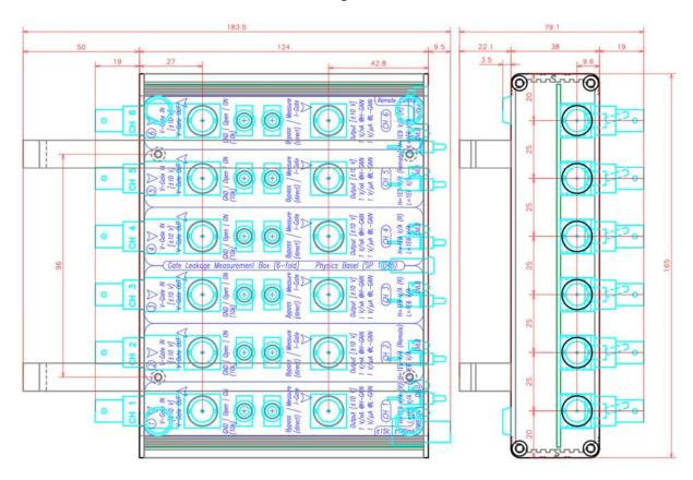
The mechanical channel to channel spacing is 25 mm which is compatible to the LNHR DAC. The total weight of the device is about 1 kg.
