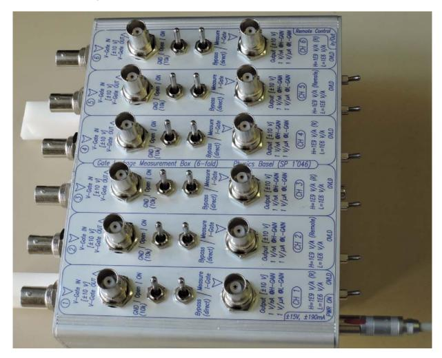
While measuring the leakage current (toggle switch in the position Measure I-Gate) the maximum DC gate current gets restricted by the GLMB to  $\pm 25$  nA in HIGH-gain respectively to  $\pm 25$   $\mu$ A in LOW-gain range. This gives some protection to the sample and the wiring of the cryostat.
