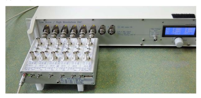
The mounting set consist of six BNC plug-to-plug adapters (length = 31.5 mm, Cinch 27-8130), two isolating plastic mounting rails and four M3-screws (length = 25 mm).
