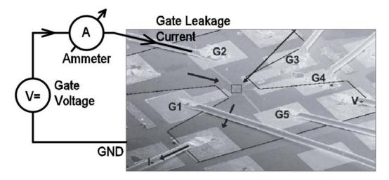
To overcome all these problems the Gate Leakage Measurement Box (GLMB) has been developed at the Physics Department of the University Basel. During an ongoing experiment, up to six gate leakage currents can be measured in parallel without strongly degrading the quality of the gate voltages.
