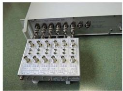
3. Insert the BNC connectors of the GLMB to BNC adapters and press the box until the BNC connectors are completely inside and the two mounting rails touch the front panel of the LNHR DAC; perhaps you have to wiggle the GLMB slightly. Now fix the BNC adapters on the GLMB side by turning them counter-clockwise until they are all locked:
