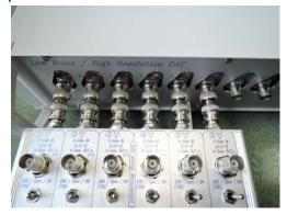
4. Power on the GLMB and switch on the LNHR DAC; now you can start cabling your setup. The not occupied DAC outputs channels 7 and 8 can be used for other purpose. The tandem-pair (GLMB and LNHR DAC) can be operated on the table (photo left) as well as inside a 19"-rack (photo right):
