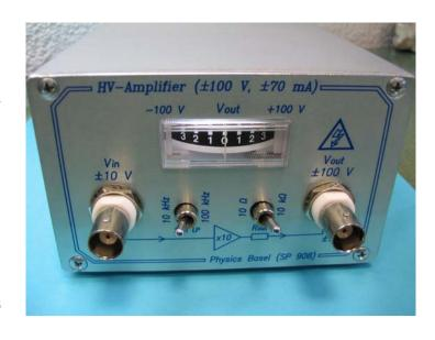
The output resistance can be chosen between 10  $\Omega$  (for low impedance loads) and 10  $k\Omega$  (for high impedance loads). The internal short-circuit protection limits the maximum output current to  $\pm 100$  mA. Nevertheless, do not short-cut the output for a longer time; it could damage the device. If short-cuts are feasible in your application, switch the output resistance to  $10~k\Omega$ ; this limits the maximum short-cut output current to save  $\pm 10~mA$ .
