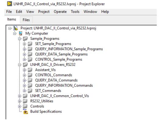
The folder "Sample Programs" is structured in SET, QUERY\_INFORMATION, QUERY\_DATA and CONTROL sample programs. After unfolding the "SET\_Sample\_Programs" one can the desired **SET** sample program open (e.g. the "Sample\_Program\_SET\_DAC\_Voltage\_ARRAY\_RS232.vi"):
