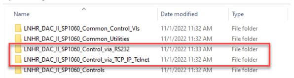
It is recommended to use the TCP/IP-Telnet communication to the LNHR DAC II as it is much faster and less prone to interference.
