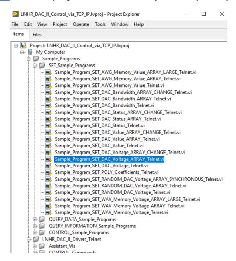
Before you start this sample program select the number of DAC-channels (12 or 24) and choose the same "TCP/IP-Address" as set on the LNHR DAC II (see local LCD under "TCP/IP Settings"). Connect the LAN Ethernet port (configured as private network) of your computer to the LAN Ethernet port on the back-panel of the LNHR DAC II by using a LAN cable (minimum Cat 5e). For details see the chapter "Communication via TCP/IP-Telnet Port" in the documentation "LNHR\_DAC\_II\_Programmers\_Manual".
