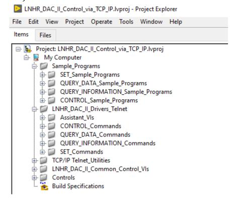
folder "Sample\_Programs" is structured in SET, QUERY\_INFORMATION, QUERY\_DATA and CONTROL sample programs. After unfolding "SET Sample Programs" one can open the desired SET sample program (e.g. the "Sample Program SET DAC Voltage ARRAY Telnet.vi"):
