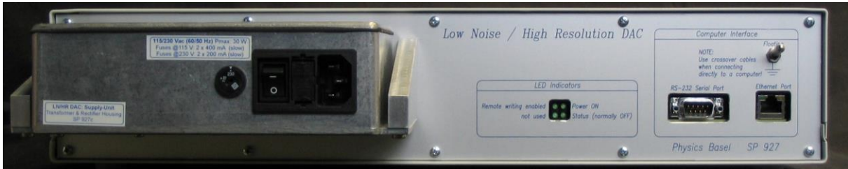
Photo 2: The rear-panel of the LNHR DAC with the attached Transformer & Rectifier Housing on the left.
