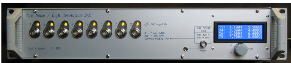
Photo 1: The front-panel of the LNHR DAC with all DAC channels switched on.
