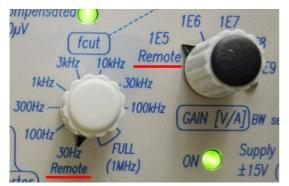
While using the remote control interface it is important that the two rotary switches on the *LNHS I to V Converter (SP 983)* are set to the position "Remote" (see photo on the left). The *GAIN [V/A]* has to be in the position "1E5, Remote" and the fcut must be set to the position "30Hz, Remote"; both knobs are then in its most counter-clockwise position.
