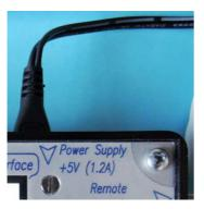
The included wide input (100...240 VAC) wall-plug power supply (HNP10I-microUSB, 5 V, 2 A) has to be connected to the remote control interface on the top right side (see left).
