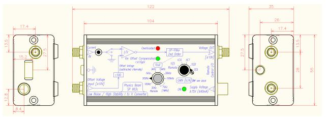
The size [mm] and position of the connectors are shown above. The weight of the device is only 165 g.
