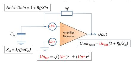
When loading an I/V converter at its input with the impedance  $(X_{in})$  the total input voltage noise  $(Un_{tot})$  is amplified by the *Noise Gain* =  $1 + Rf/X_{in}$ . Herby the assumption is made that the differential amplifier has an infinite voltage gain.
