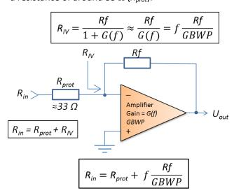
For AC signals the input resistance  $(R_{in})$  is increased by the virtual input impedance  $(R_{IV})$  of the I/V converter which is depended on the frequency (f), the feedback-resistor (Rf = gain) and the gain bandwidth product (GBWP) of the amplifier (see left). The GBWP of the LNHS I/V Converter is about 600 MHz.
