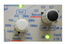
When the gain is remote controlled the rotary switch "GAIN" has to be in the position "1E5, Remote". For remote controlling the LP-filter cut-off frequency the rotary switch "fcut" must be set to the position "30Hz, Remote" (see left). It is possible to control only the gain or only the cut-off frequency remotely and manually set the other by the rotary switch.
