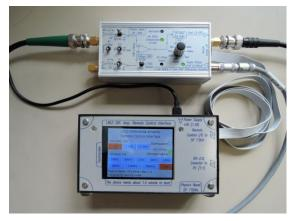
When using the *Remote Control Interface (SP 1'004a)* – shown on the left – the parameters can be adjusted manually (touch-screen) or via simple ASCII commands send form a computer via a serial interface (RS-232) at a baud-rate of 9'600.
