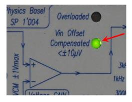
The green LED *Vin Offset Compensated* lights up when the input offset voltage gets stabilized within around  $\pm 10~\mu V$  (see left). After power up the device it takes several minutes (typical 5...15 minutes) until the automatic input offset compensation is completed and the green LED is turned on. The entire warmup of the device takes around two hours.
