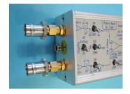
All the analog I/O signals are connected by SMA connectors to the preamplifier. If BNC connectors are preferred the stable SMA/BNC-adapters (which are included) can be screwed directly onto the *LNLD Diff Amp* (see photo on the left).
