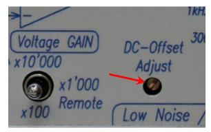
Since this offset adjustment sets the zero-voltage of the servo control loop, it reacts very slowly. Therefore perform the adjustments very gently! Make at maximum a quarter-turn and wait until the output voltage has stabilized again, before continuing the adjustment. When turning too fast, the green LED *Vin Offset Compensated* will go out.
