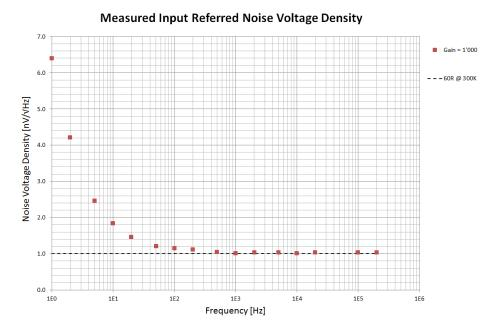
The measured integrated input noise voltage is given below; for reference also the integrated noise voltage of a 60 Ohm resistor at 300K is shown in black. The integration starts at a frequency of 0.5 Hz. For a brick-wall bandwidth from 0.5 Hz up to 1 kHz the integrated input noise voltage is around 35 nV<sub>RMS</sub> and from 0.5 Hz up to 100 kHz around 310 nV<sub>RMS</sub>.
