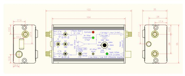
The size [mm] and position of the connectors are shown above. The weight of the device is 286 g; this allows the mounting directly onto the breakout-box of the cryostat.
