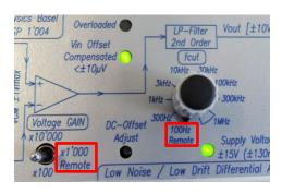
When the gain is remotely controlled the switch "Voltage GAIN" has to be in the position "x1'000, Remote". For remote controlling the LP-filter cut-off frequency the rotary switch "fcut" must be set to the position "100Hz, Remote" (see left). It is possible to control only the gain or only the cut-off frequency remotely and manually set the other by the switch.
