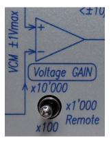
The voltage gain of the *LNLD Diff Amp* can be switched over the following three decades: x100, x1'000, x10'000 corresponding to a maximum input voltage of  $\pm 100$  mV,  $\pm 1$  mV. These ranges cover the most often used gains in cryogenic experiments. The accuracy of the voltage gain is typical better than  $\pm 1\%$  (max.  $\pm 3\%$ ).
