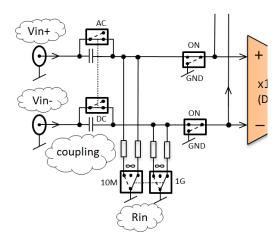
The *Vin+* is the NON-INVERTING voltage input while the *Vin*-is the INVERTING voltage input of the differential amplifier (see left).
